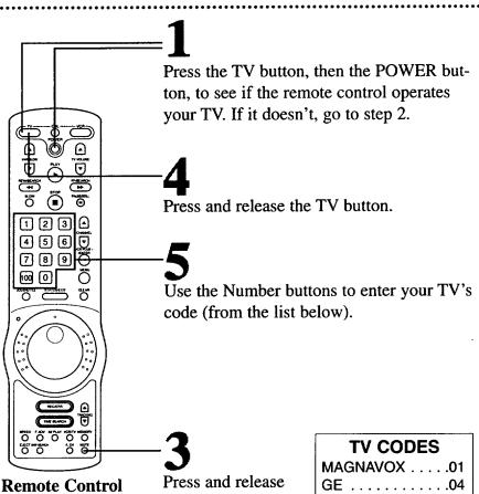
**D** Try step 1 again. If the remote control works your **T**V, you're finished. If the remote control still doesn't work your TV, repeat steps 2 - 5 using another code.
